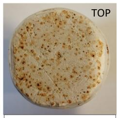
Fig. 1: Chalk core (1.5 inch) after polymer injection. The polymer is orange/brown color and can be observed at the top of the core, demonstrating that it has gone through the core matrix.
