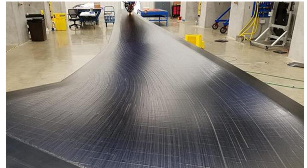
Aircraft wing manufactured with tow steering, credit: Aurora Flight Sciences
