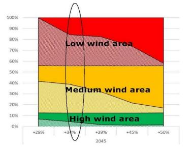
Shaded areas show the predicted share of LowWind technology of the windturbine market in 2045 as a function of increased CapEx relative to the cost of conventional turbine technology.
