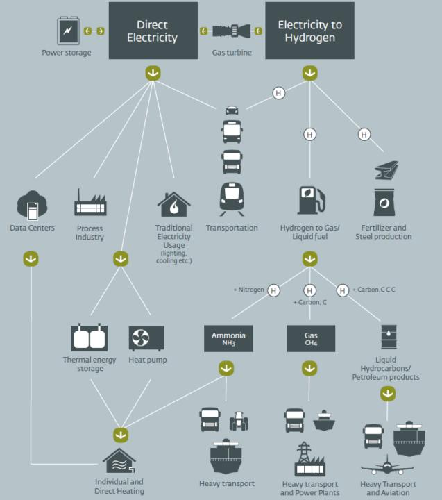
Power to X - from electrons to hydrogen-based electrofuels
