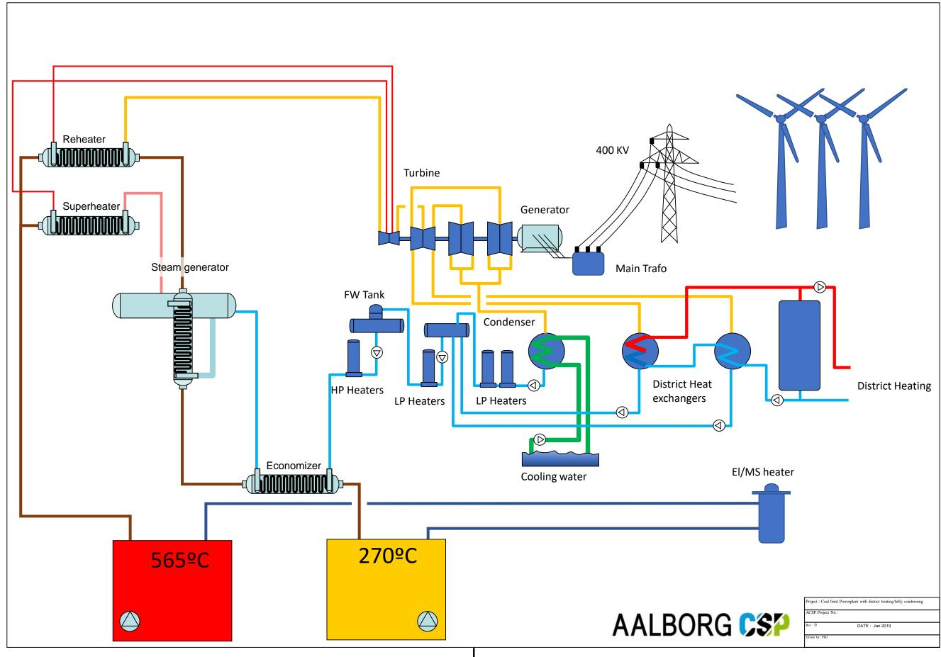
Typical reuseable assets from converted Coal fired power plant
